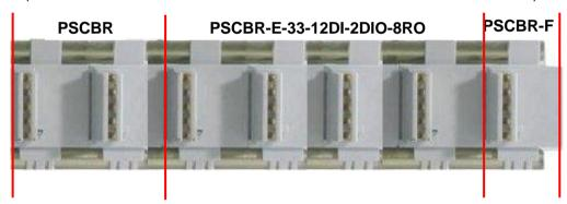
Power supply for PSCBR-E-33-12DI-2DIO-8RO module is on the back plane bus and is generated from basic device.
